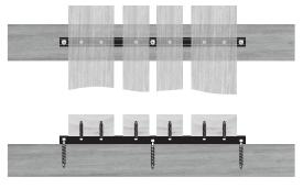
The wooden battens are fixed at the back with one or two screws, depending on the width of the batten. The fixing to the sub-structure is carried out between the wooden battens.
