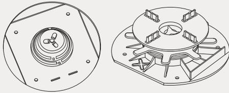
Pre-marked cutting lines for easy base plate resizing
