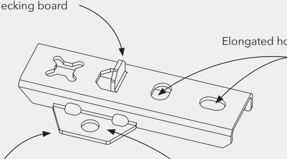
Elongated holes for precise positioning and position correction
