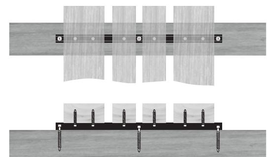
The wooden battens are fixed at the back with one or two screws, depending on the width of the batten. The fixing to the sub-structure is carried out between the wooden battens.
