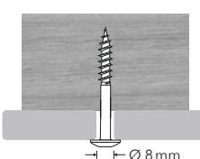
The **sliding points** accommodate dimensional changes in the facade panel. The facade screw is screwed in flush, allowing the panels to move freely.
