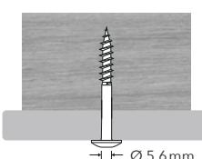
The **fixed point** secures the facade panel in place; its positioning can vary between manufacturers.
