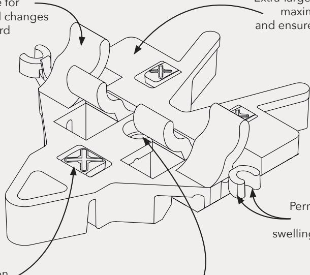
Extra-large base plate provides maximum bearing surface and ensures perfect ventilation
