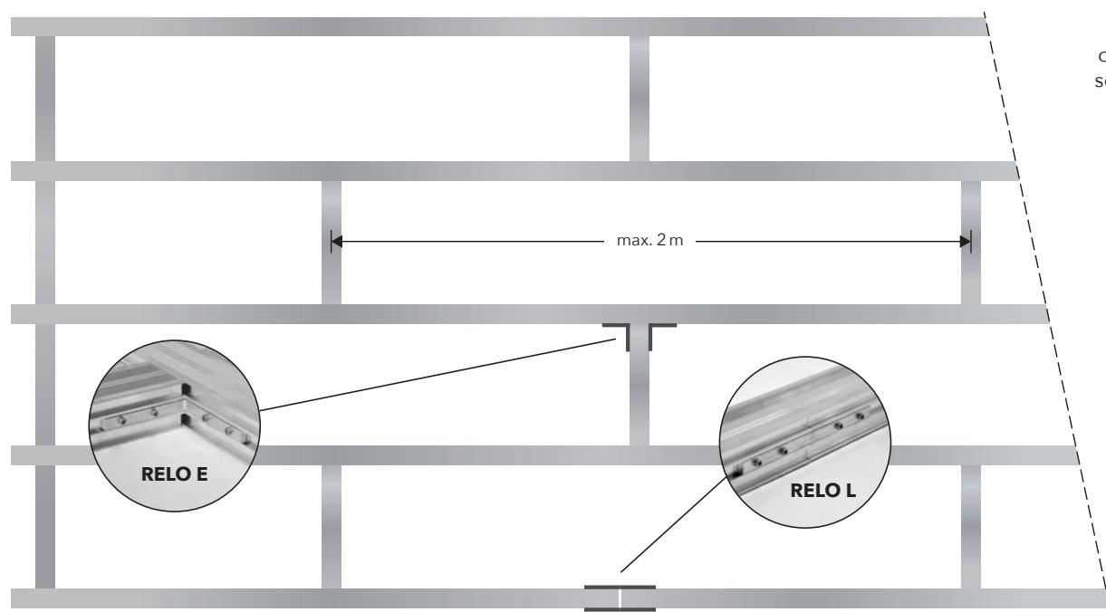
RELO frame construction with securely fastened corner and lengthwise connections.
