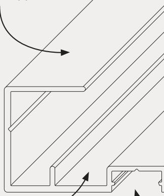
Insert Channel: Accommodates FUGO joint spacers seamlessly
